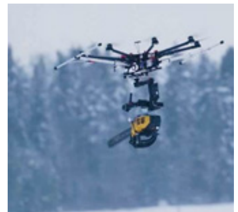
Yes, it's real: A remote-controlled chainsaw drone. ( https://www.youtube.com/watch?v=6Viwwetf0gU ). Photo permission courtesy of Noodletail Videos)
